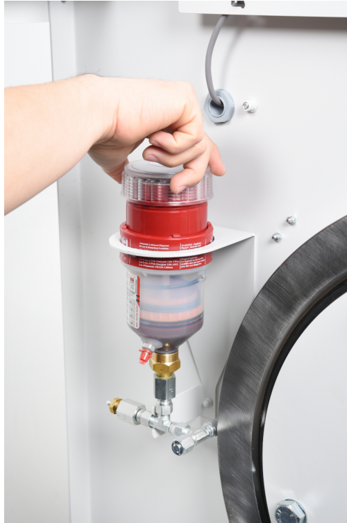
Figure 77. Removing the top cap of the lubricator
