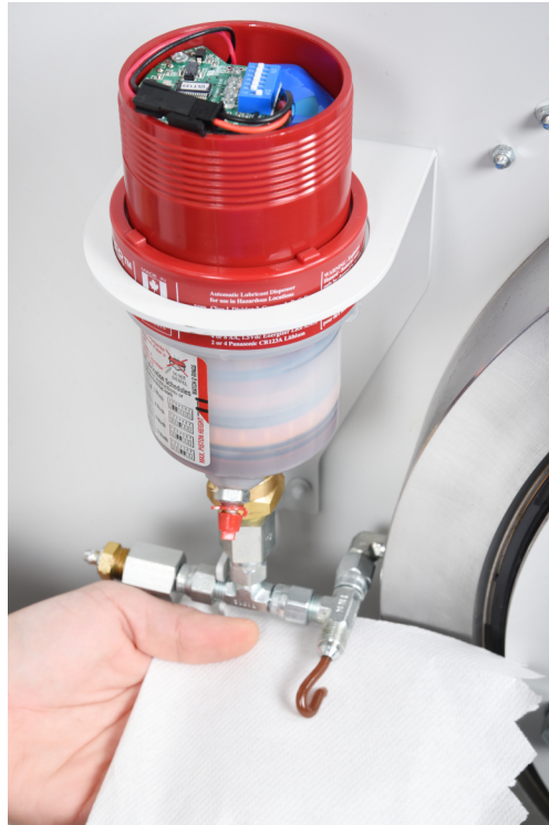
Figure 79. Lubricator dispensing grease.
