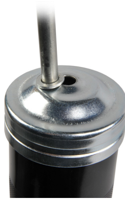
Figure 64. Locking the rod handle.
