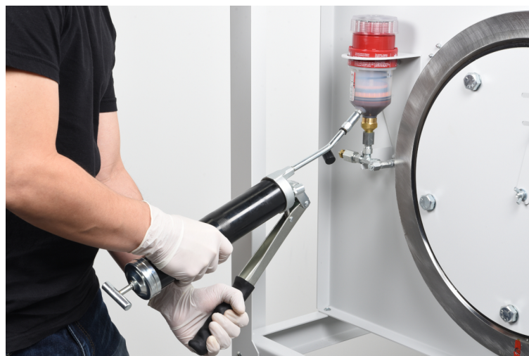
Figure 76. Pumping a small amount of grease inside the automatic lubricator
