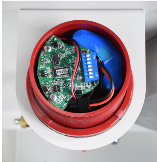
Figure 63. DIP switches on the automatic lubricator
