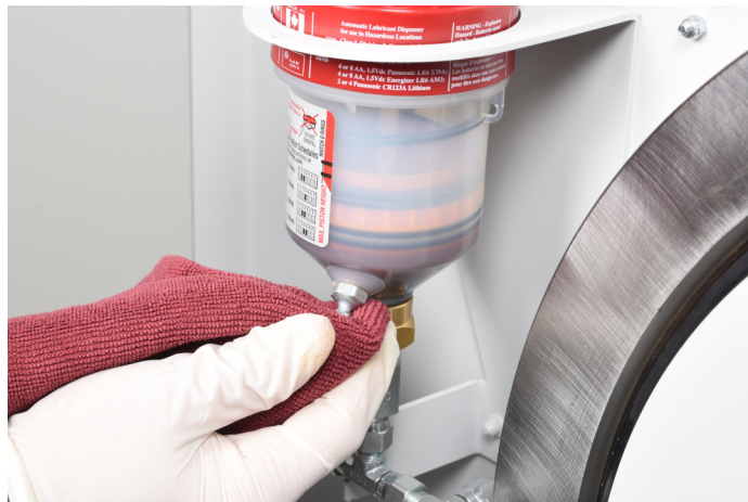
Figure 74. Cleaning the lubricator grease fitting.
