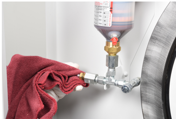
Figure 71. Cleaning the slewing bearing grease fitting.
