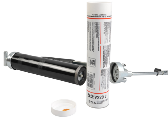
Figure 66. Removing the plastic cap.
