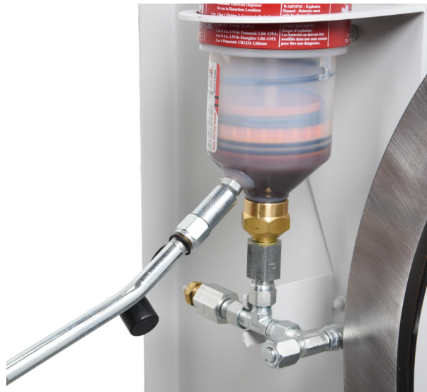
Figure 75. Inserting the grease gun into the lubricator grease fitting.
