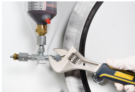
Figure 70. Removing the bleed plug.
